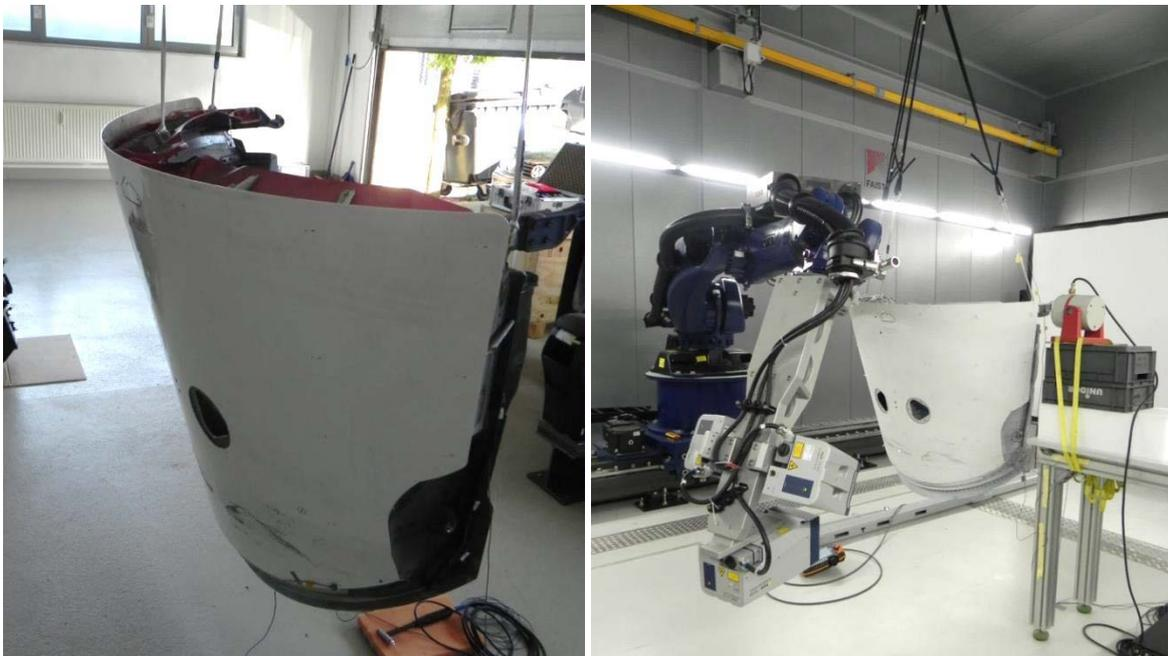
Figure 14: Typical test setup, left: conventional hammer test, right: automated 3D laser scanner (RoboVib)
