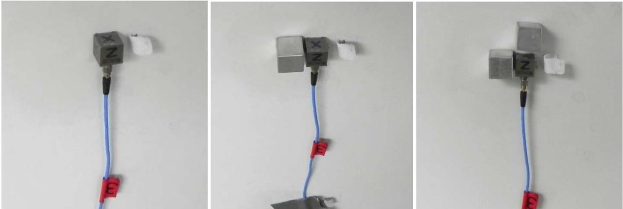
Figure 12: Mass loading setup
