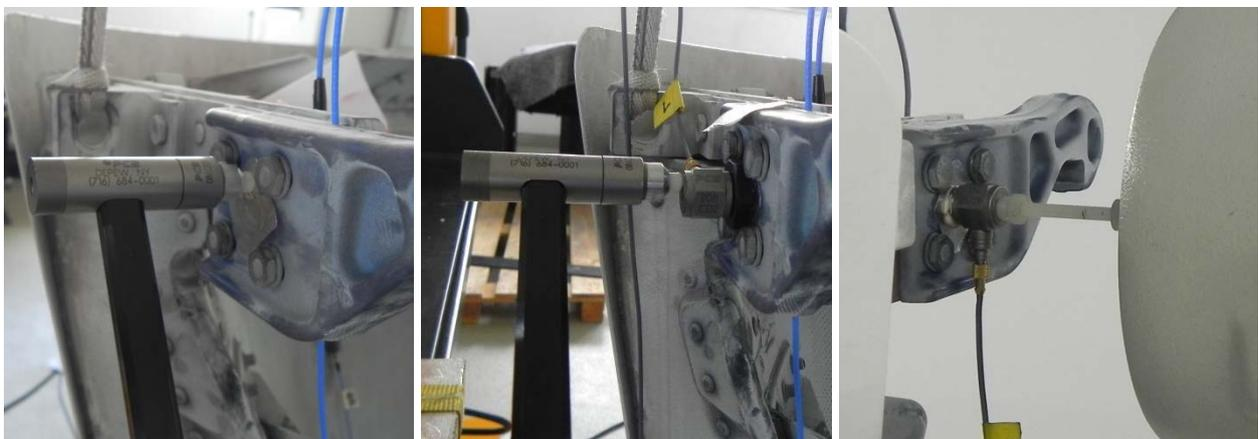
Figure 9: Configurations for stinger/force sensor attachment investigation
