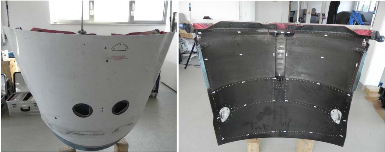
Figure 1: Survey of TRU door, left: outer, right inner view
