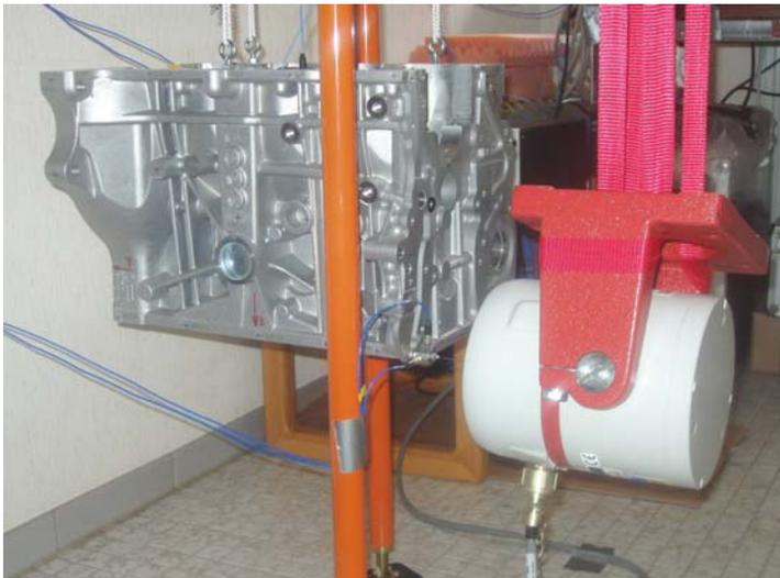
Figure 7: Test setup with modal exciter
