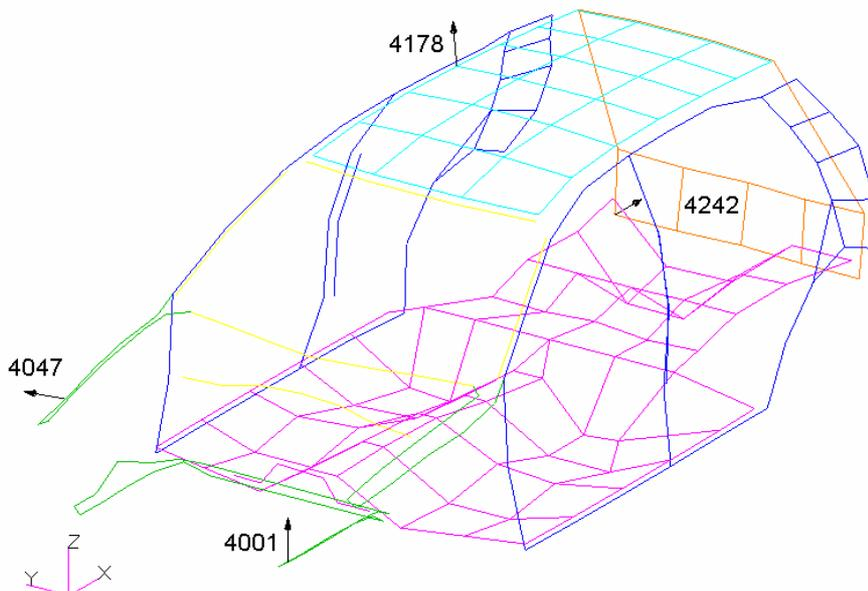
Figure 6: Test model of the body in white with exciter degrees of freedom
