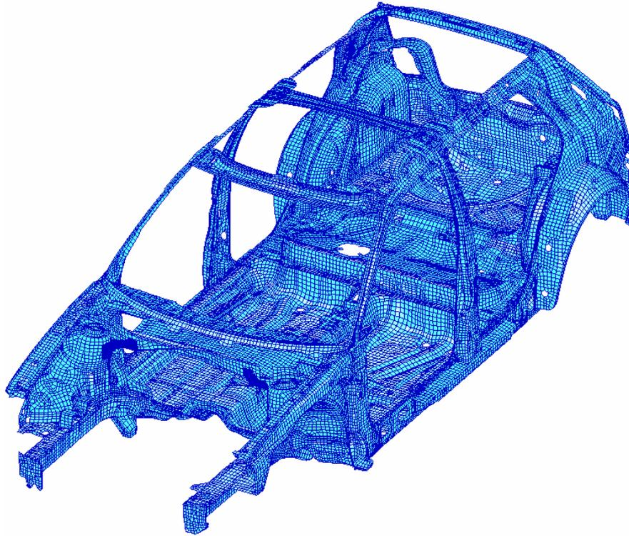
Figure 2: Finite Element model of the body in white
