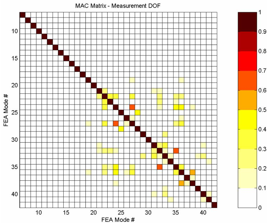
Figure 4: Auto MAC matrix of analytical mode shapes at measurement degrees of freedom
