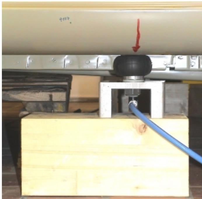
Figure 7: Mounting of the body in white using air springs
