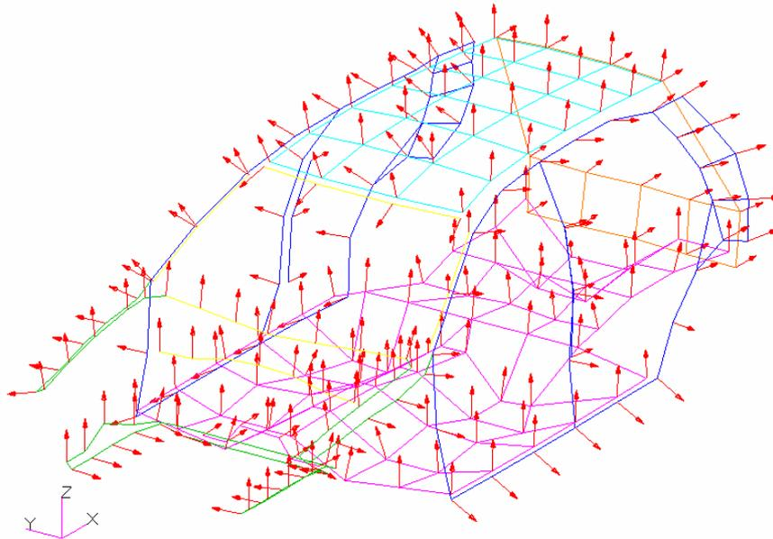
Figure 3: Test model of the body in white with measurement degrees of freedom
