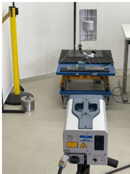
Figure 11: Measurement setup with 1D laser scanner and automatic hammer excitation
